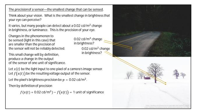
The precisoin of a sensor—the smallest change that can be sensed.
