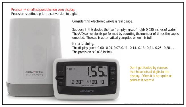
The dynamic range of a sensor—number of distinguishable levels.
